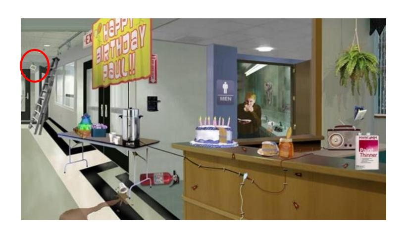
Passageway by the counter has an electric cord hung across it. Aisles and passageways shall be kept clear and in good repairs, with no obstruction across or in the aisles that could create a hazard.
