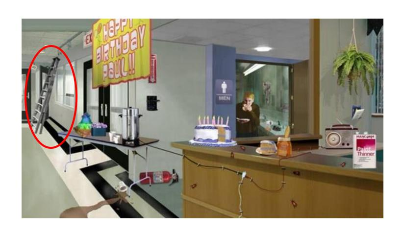
Fire extinguisher is on the floor instead of in its designated place. The employer shall assure that portable fire extinguishers are maintained in a fully charged and operable conditions and kept in their designated places at all times except during use.
