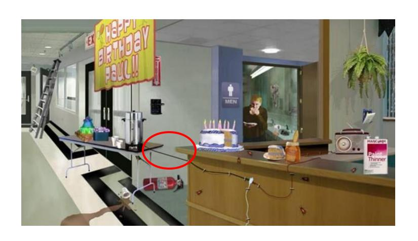
Wiring is exposed below the hanging plant. Water could drip down from the plant. Receptacles may have no live parts normally exposed to employee contact.
